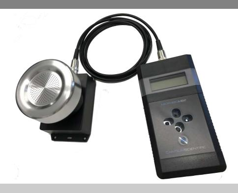
Bioaerosol samplers are vital equipment for use in bioaerosol research, clean rooms, pharmaceutical validation and throughout hospitals wherever air hygiene is paramount. The MicroBio MB2-RSH Bioaerosol Sampler has a host of features making it ideal for use in applications from isolator cabinets to sealed clean rooms and production cells.
