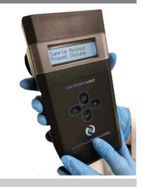
Bioaerosol samplers are vital equipment for use in bioaerosol research, clean rooms, pharmaceutical validation and throughout healthcare wherever air hygiene is vital. Designed to meet the requirements of ISO14698 and ISO17141, the MicroBio MB2 Bioaerosol Sampler has a host of features making it ideal for use in such applications.
