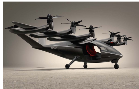
Fig. 8. Archer Maker eVTOL with fixed rotor for lift and tilt-rotor for vectored thrust [34].
