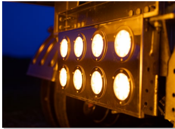
Forward facing bogie lights in a stainless steel box
