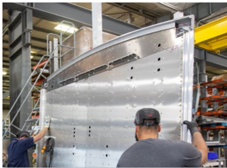
Integrated arched headers & cast aluminum corner caps come standard for added strength and style, eliminating out-dated bolt-on tarp caps.
