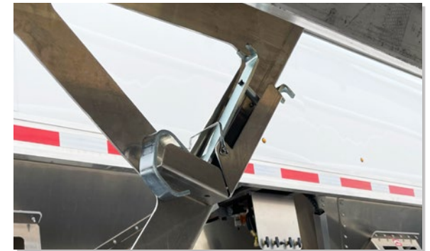
Industry exclusive removable manual tarp crank retainer bar stored on curbside dolly leg gusset for emergency access. Can be installed without tools.
