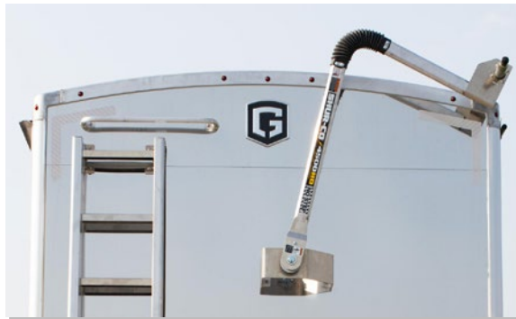
New horizontal seam design on front and rear panels. Cleaner appearance and less panel distortion.
