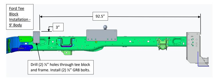
The view above shows an F350. For F450 and F550, flip the tee block around so that the small flange is facing outwards. Locate the tee block vertically and horizontally as shown and drill (2) ½" holes through the tee block and frame. Install (2) ½" GR8 bolts, using ½" washers as shims to level the tee block.
