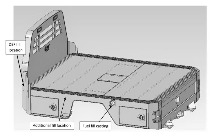
Route the fuel fill hose and neck up to the fuel fill casting and attach the filler neck to the casting.
