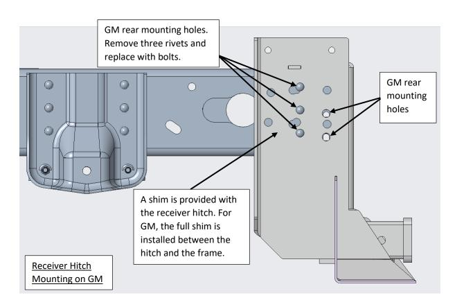
Install the gooseneck hitch at the dimension shown below. Drill (4) ½" holes, per side, through the chassis frame, using the hitch as a guide. Prior to drilling any holes referenced throughout this procedure, check that the holes will not interfere with or damage any components on the chassis. Install ½" grade 8 bolts and nuts in the gooseneck hitch holes.
