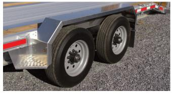
Heavy-duty steel wheels with two 10K Dexter torsion ride axles to handle whatever you need to haul
