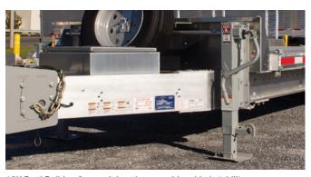
12K Dual Bulldog 2-speed drop-legs provide added stability
