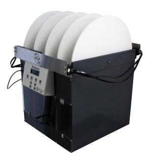
The drum texture is critical to the proper operation of a rotarod. The Rotamex-5 employs a special surface treatment for optimal grip and easy cleaning.
