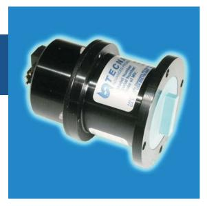
Using the magnetic coupling technology developed for Tecnadyne's underwater thruser motors, the Model 194 places the sensor in a hermetically sealed housing with no rotating shaft seals that can leak and cause failure.
