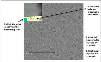
**Figure 3.** Example of the NIS measurement tool. This will come up in a new window when you left-click on any image in the viewer.
