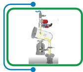
The dip-pipe is N2 flushed to drain the system
