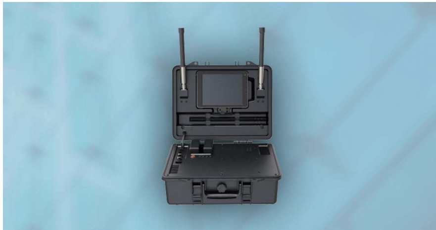
Figure 42 - A mobile Aeroscope unit used during Nozomi Networks Labs experiments, consisting of an Android tablet with dedicated USB hardware.
