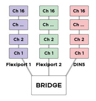
Example: Output the first 16 messages from Flexi 1, the second 16 from Flexi 2, and the third 16 from the DIN5 MIDI out. By using all 16 MIDI channels on each output (message 1/channel 1, message 2/channel2) this will result in 48 different devices able to be MIDI controlled by a single footswitch press with no conflicting MIDI channels.
