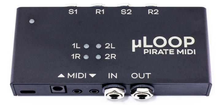
4 mono loops or 2 stereo loops in an enclosure that fits under the smallest pedalboards - only 22mm thick. Plus a USB MIDI Interface!
