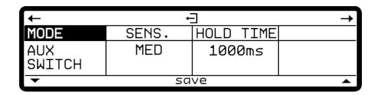
Aux Switch sensitivity is a setting designed to accommodate different brands of switches that might physically differ in the way their switches behave. The sensitivity is something you can change if you are noticing erratic behaviour of your Aux Switch.
