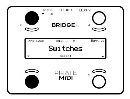
Press **switch 1 or switch 2 to navigate the menu** (note the arrows on screen).
