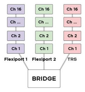
(message 1/channel 1, message 2/channel2) this will result in 48 different devices able to be MIDI controlled by a single footswitch press with no conflicting MIDI channels.
