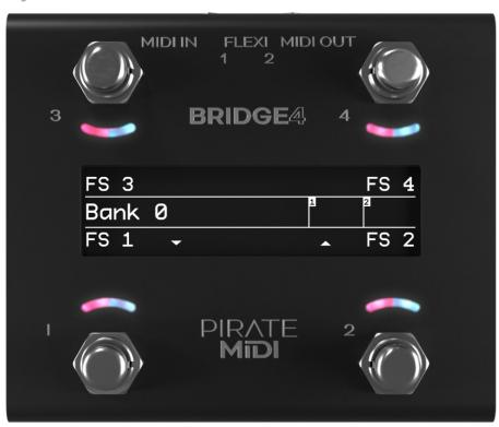
The **BRIDGE4** is a 4-switch MIDI foot controller with RGB LEDs, an OLED screen, and a super tough aluminium enclosure. It's made in New South Wales, Australia and was the result of a successful Kickstarter campaign in 2020.
