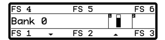
Switch labels and bank name are still visible, but they are slightly smaller, and the bank name is left aligned. The bank up and down indicator icons are also present.
