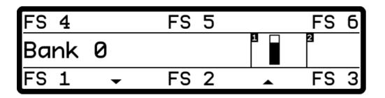
Switch labels and bank name are still visible, but they are slightly smaller, and the bank name is left aligned. The bank up and down indicator icons are also present.
