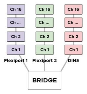
(message 1/channel 1, message 2/channel2) this will result in 48 different devices able to be MIDI controlled by a single footswitch press with no conflicting MIDI channels.
