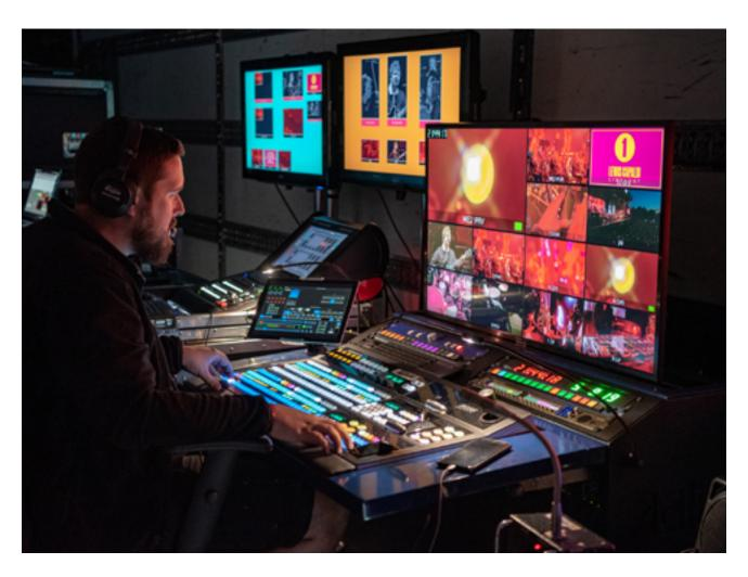
All screens were Unilumin UPADIIIH05 with Novastar processing and Barco E2 / EC30 for screen management. The camera system comprised 4 x Sony HD camera channels (2 at FOH with Box Lenses) and Ross Carbonite PPU. Playback was handled by Resolume and QLab media servers.
