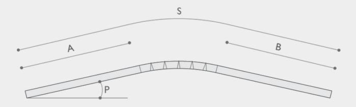
A sheet curved exclusively at its center to create the ridge and connect two slopes, accomplished by employing a series of indentations in the middle of the sheet. The length of the straight sections A and B ranges from a minimum of 175 mm to a maximum of 4000 mm
