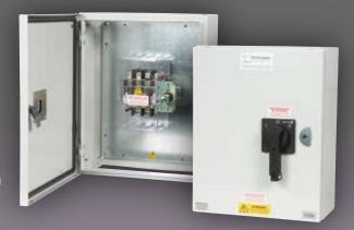
PLEASE NOTE: Changeover switch should be selected to match the current taken by the load being supplied. In the absence of this information select based on the higher current of the supplies. If using a generator it is unreliable to use its kVA rating to calculate changeover switch size.
