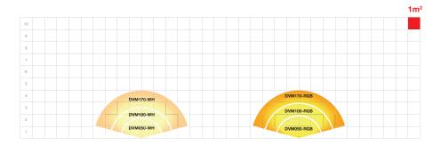
Values in graph refer to swimming pools with white or light-coloured walls that require  $100-150 \text{ lm/m}^2$ . Increase the light (lumen) by 50% for medium colours. Dark walls are difficult to illuminate and need up to 250% extra light.
