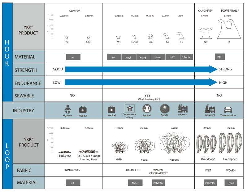
$\label{eq:polymer} \textbf{PP} = \textbf{Polypropylene} \quad \textbf{Vinyl} = \textbf{PVC} \ (\textbf{Polyvinyl Chloride}) \quad \textbf{HDPE} = \textbf{High-Density Polyethylene} \quad \textbf{PBT} = \textbf{Polybutylene Terephthalate}$
