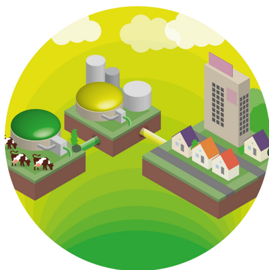
Figure 8.3 Biogas distribution system supplemented where necessary by natural gas injection (Source RVO; Netherlands)
