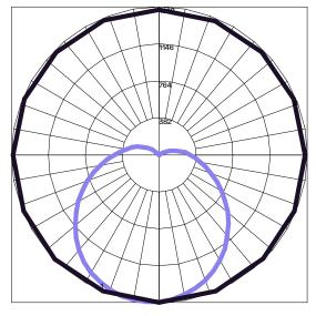
Maximum Candela = 1528.3 Located At Horizontal Angle = 270, Vertical Angle = 5 # 1 - Vertical Plane Through Horizontal Angles (270 - 90) (Through Max. Cd.) # 2 - Horizontal Cone Through Vertical Angle (5) (Through Max. Cd.)
