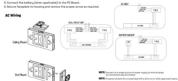
WARNING: Unused wires must be capped using enclosed wire nuts.
