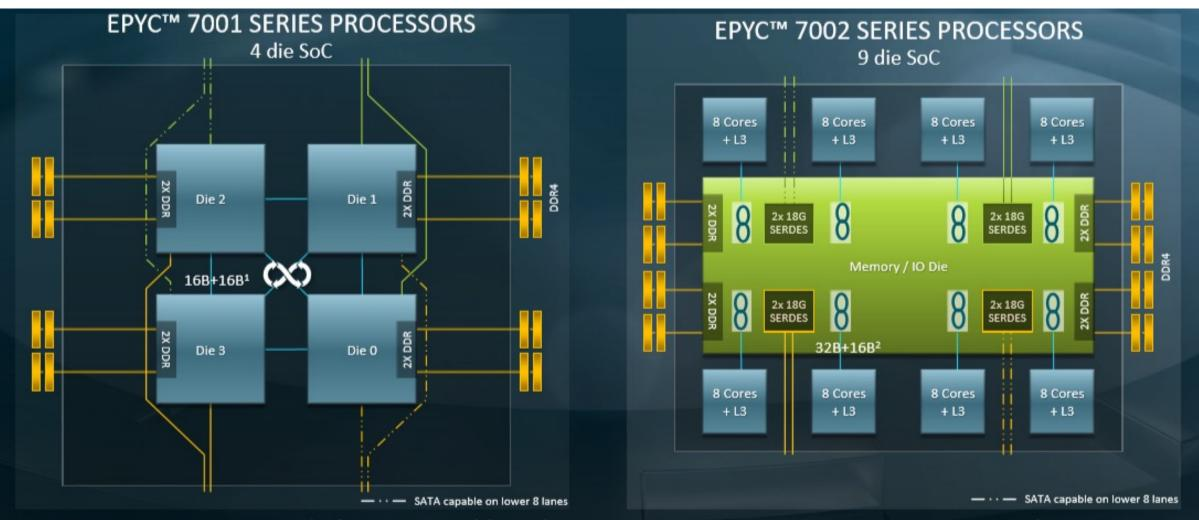
EPYC<sup>™</sup> 7002 Series is Platform Compatible with EPYC<sup>™</sup> 7001 Series to Optimize Ecosystem Deployment Performance-optimized Die-to-die Infinity Fabric<sup>™</sup>
