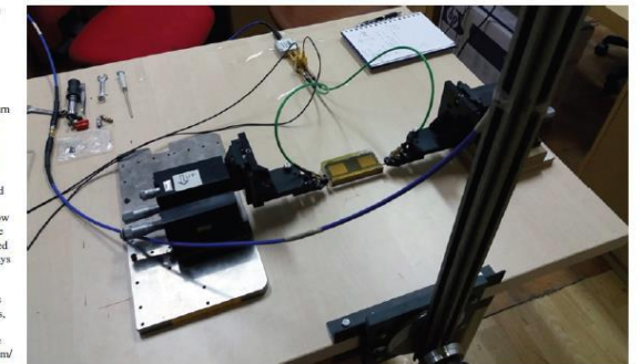
TOP: RF testing measurement setup of the HfZrO 2 -based phased antenna array that was characterised at IMT. BOTTOM: Detail of the bias circuit for the phase shifters in the HfZrO 2 -based phased antenna array
