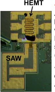
• SAW-HEMT sensor structure: an AlGaN/GaN heterostructure, grown by MOCVD on (111) Si substrates, was used to fabricate on it a power HEMT and a SAW to demonstrate in situ power transistor heat monitoring (for monolithic integration)
