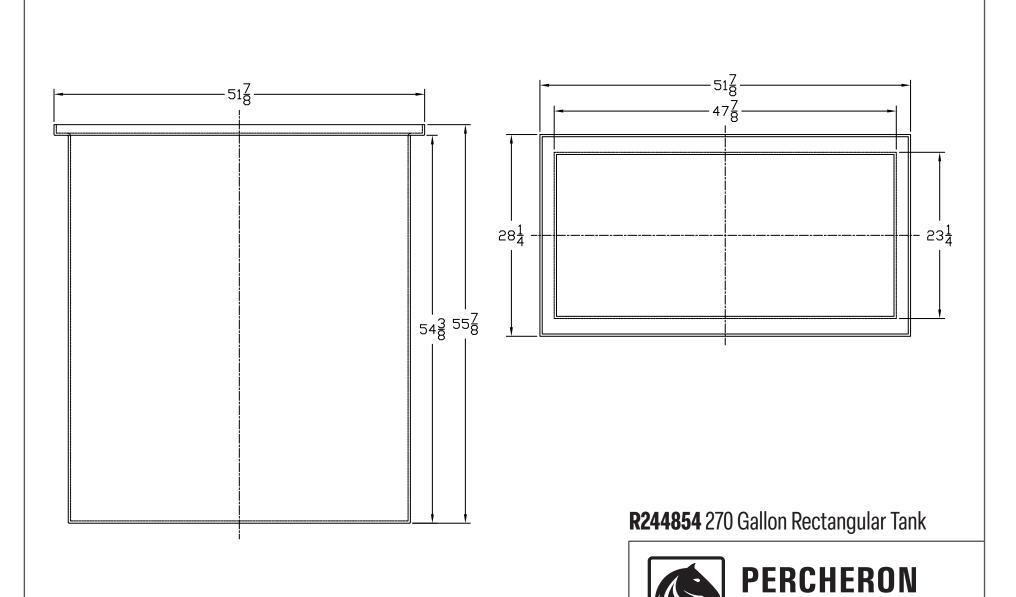
All dimensions shown are outside part dimensions in inches, and vary by the standard rotational molding tolerance of +2/-3%.
