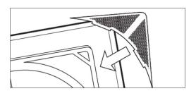
6. Place the roof assembly onto the roof tile batons. The upper end of the flashing unit should be under the roof tiles above. The bottom of the unit with the lead attached should be on top of the tile below.
