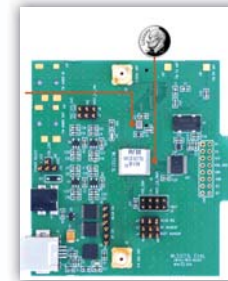
WLS1273L Module Installed on DR-WLS1273L-EV Evaluation Board
