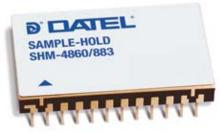
Sample-Hold Amplifiers shorten the aperture time for A/D converters by rapidly sampling the input signal and then holding its value until the conversion is completed. Many A/D converters now include the sample-hold with
