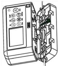
2. Press the cassette latch lock down and firmly push the cassette towards the pump.
