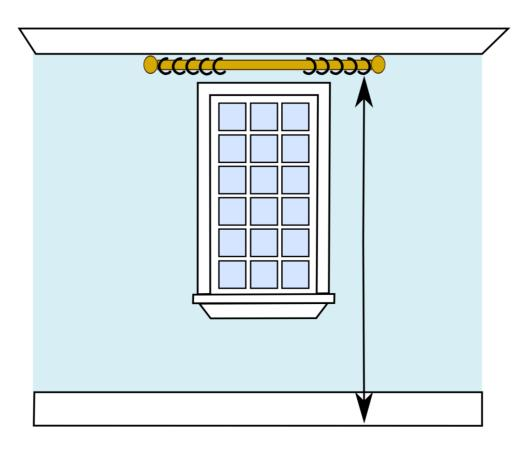
These traversing panels are a good example of when to do a Top Down Measure.
