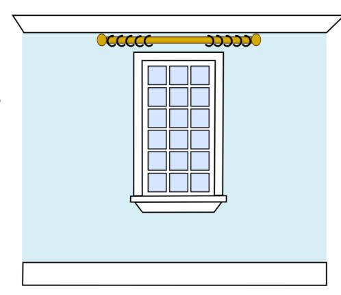
Once the hardware is installed, a measurement is taken from the bottom of the ring to the floor. Then the work order can be done and sent on to the workroom.
