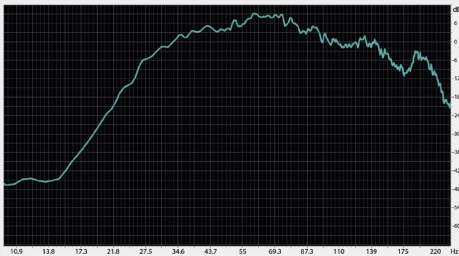
The rapid drop-off of a bass-reflex design is clear below 30Hz, but response was solid and extended above that.
