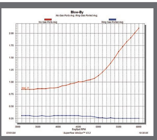
Proven increased horsepower and reduction in blow-by
