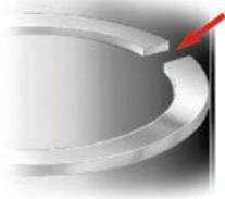
**THE END GAP** – Here is the correlation...the larger the end gap, the more blow-by and power reduction your engine will see.
