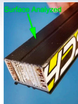
Figure 1a. Bottom surface of ski analyzed using handheld LIBS.
