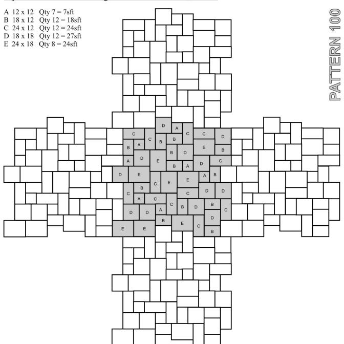
These patterns have been configured to work with STONEarch stone products. Patterns are suggestive only and may require modification as per site requirements and installation technique used. Please plan some extra stone for cutting/wastage. We are not responsible for any direct or indirect cost of installation, shipping, shortages or overages. Stone sizes are approximate, slight size variations are to be expected in natural stone.
