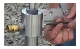
Unscrew the clevis from the pump rod using your vice grip or channel lock. Move the lever arm clockwise while keeping the pump rod from rotating. The direction you unscrew is the opposite of normal -- turn clockwise to remove, rather than the normal counterclockwise.
