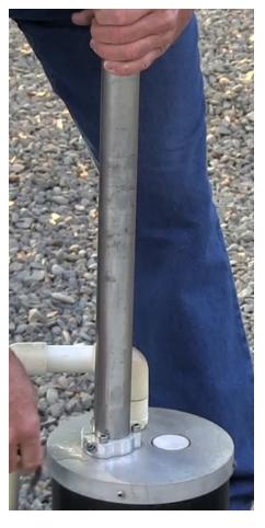
Remove the pump head by unscrewing it (below) -- rotating it in a counterclockwise motion. You may need to first loosen it with a channel lock.
