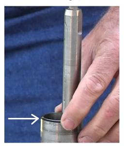
Lift the pump assembly over the riser tube...
