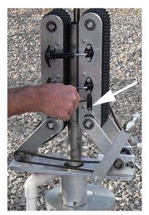
**Attach the four tensioners** (left). There are two on each side -- only two are visible in the photo (left).
