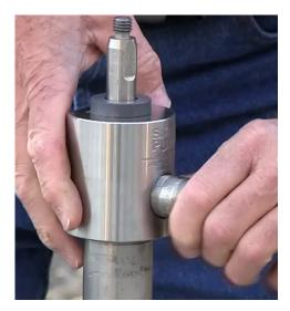
After removing the pump head, check to make sure stationary O-ring at the top of the riser tube remains there (right, white arrow).
