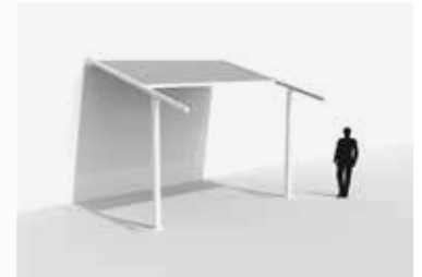
With roof overhang [with “shifted” columns]
