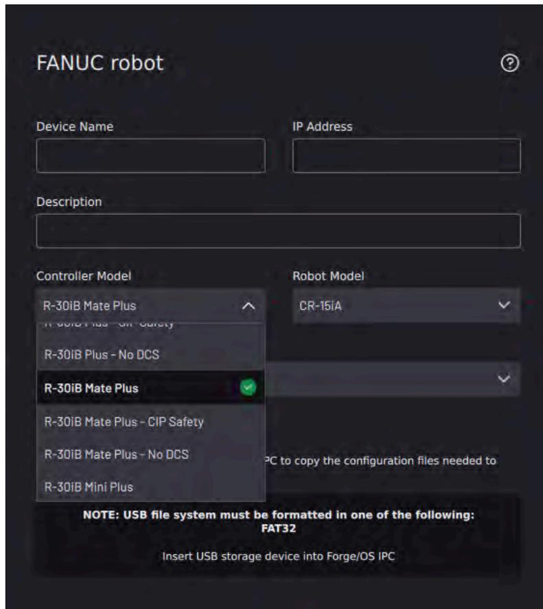
6. Insert a USB flash drive into the IPC as instructed on the screen. Use an empty flash drive with at least 2GB of storage.
