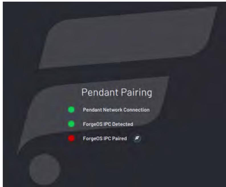
The UI shows the real-time state of each step. For example, if the pendant loses its network connection during pairing, all steps become undone.
