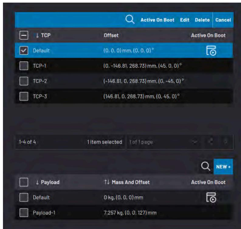
4. Tap **SAVE** to exit the robot configuration. Forge/OS uploads the tool data to the FANUC controller. Forge/OS shows an error for the robot: *FANUC Error SYST-212: DCS settings not applied.*
