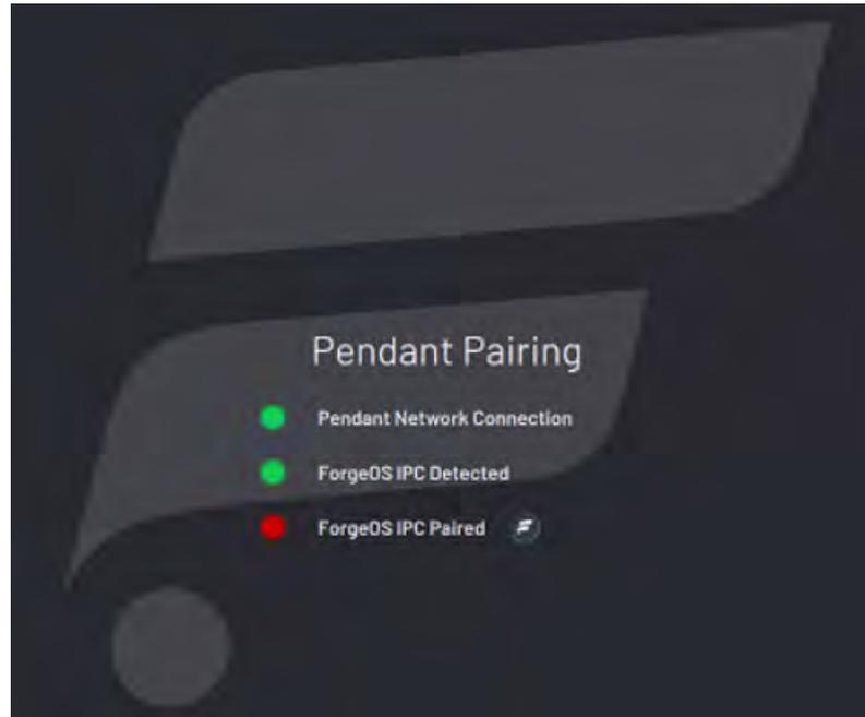
The UI shows the real-time state of each step. For example, if the pendant loses its network connection during pairing, all steps become undone. If the READY pendant spends more than 60 seconds on any step, troubleshooting text displays. Common things to check are if the READY pendant network cable is plugged in, if the IPC is powered on, if the READY pendant and IPC are connected to the same network, and if there's only one READY pendant and one IPC on that network.
