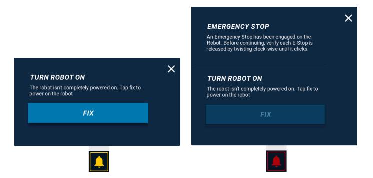
The Notification Center displaying the **FIX** button when in a Robot Warning state, and displaying the current system status when an Emergency Stop button is pressed.
