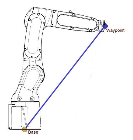
Throughout Forge, Waypoints are the most common parameter with which you will program the robot arm to move. Blocks on the canvas directing the arm to move to machine tools, iterate through a grid of parts, or curve around an obstacle will always reference Waypoints to define these motions and locations.
