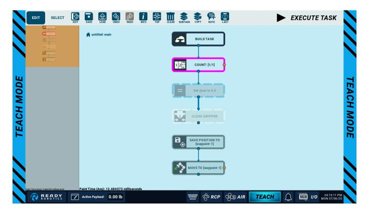
A magenta block was the Last executed in the Task. The following two blocks are ghosted because the variable and gripper are not present. The last two blocks are detached because there is no path connecting them to the Root Block.
