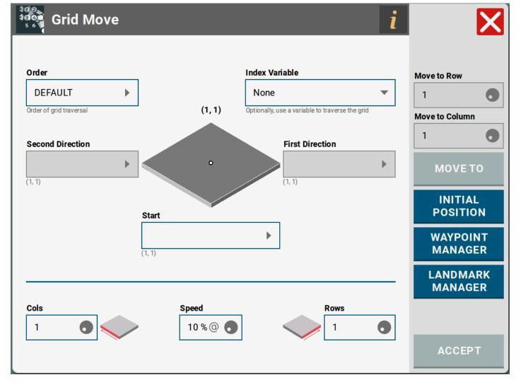
Below is the Grid Move generator that pops up when the adding a Grid block
