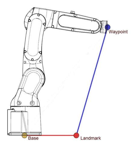
In Forge, Landmarks belong to the Task in which they were created. You can also promote a Landmark to a "shared/" Landmark which will enable you to reference it in multiple Tasks. When you change a shared/ Landmark, its pose and any Waypoints that reference it will update in any Task that uses it, even Tasks you aren't currently viewing.
