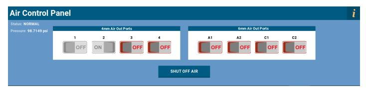
If you have pneumatic tools or devices configured to onboard air ports in Hardware Configuration, those ports will appear grayed out in the Air Control Panel.
