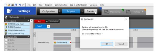
If the safety controller fails to connect, make sure it is powered on and check the USB cable to your PC.
