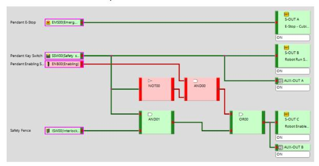
When only the E-Stop and Enabling Switch are green (closed circuits), the robot can be jogged at the reduced **Teach speed**.
