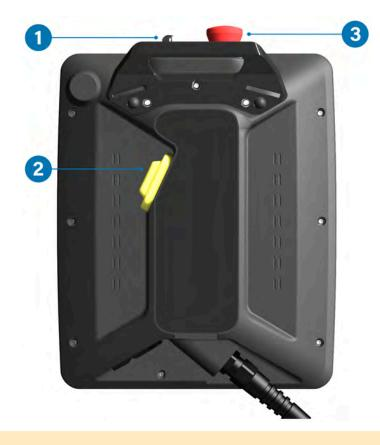
**Note:** You'll connect the **READY pendant** Emergency Stop to the UR controller. The UR robot won't use the **READY pendant** key selector switch or the three-position enabling switch. You can connect the three-position enabling switch if you configure Polyscope to use an enabling device.
