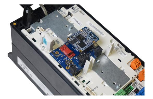
B&D developed our remote I/O option card in conjunction with SoftPLC as a means to offer customers more options and fits standard in any ABB AC or DC drive. Our option is far quicker and massively less expensive than the alternative solution from the original PLC manufacturer.
