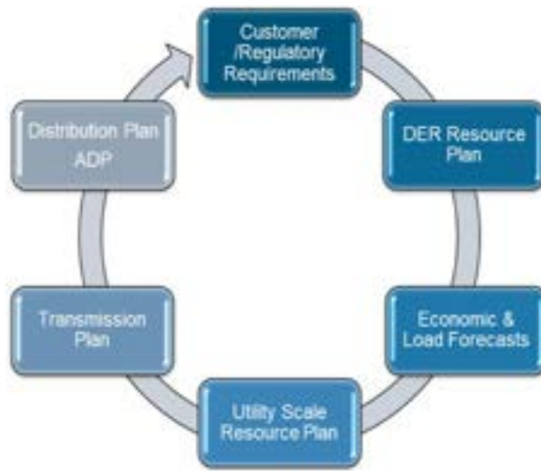
Figure 3 Integrated planning spans resource, transmission and distribution planning into a single planning process.
