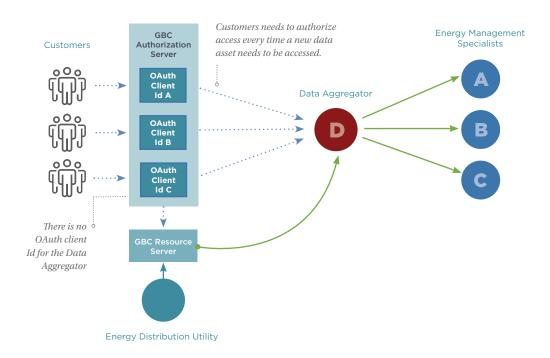
**FIGURE 9B.** Concept diagram for "Cascading" Green Button Connect OAuth 2.0 authorization. Authorization is facilitated by the Energy Management Specialists, using their OAuth Client Ids A, B, and C. Customers delegate permissioning rights to Energy Management Specialists, who pass on access rights to a Data Aggregator as needed to access data using their own OAuth Client id D.
