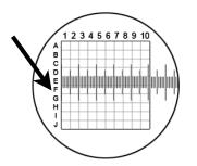
Line up one of the larger lines on the stage micrometer with the left edge of the reticle grid and measure the entire grid again. Enter this number as "Width 2" on the Scaling Factor Worksheet.
