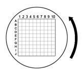
After the reticle installation, rotate the eyepiece until the grid labels are right side up and legible.
