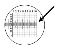
Line up one of the larger lines on the stage micrometer with the right edge of the reticle grid. Measure the distance across the row of 10 squares. Enter this number as "Width I" on the Scaling Factor Worksheet.
